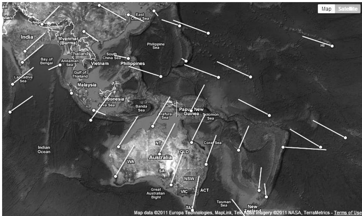
Figure 2. Displacement rates of GPS stations in the western Pacific region as compiled by JPL. (Source: sideshow.jpl.nasa.gov/mbh/series.html )
