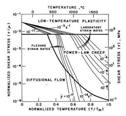
Caption: Deformation mechanism map for olivine with a 1 mm grain size. Shear strain rates  $\hat{Y}$  (in s<sup>-1</sup>) are contoured over shear stress  $\tau$  normalized by shear modulus  $\mu$  and absolute temperature T normalized by temperature of melting  $T_m$ .
