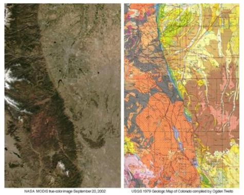
Caption: Satellite image (left) and geologic map (right) showing the abrupt transition from the Great Plains to the mountains of the Colorado Front Range. This transition involves a nearly vertical set of faults with a total vertical displacement of 15,000-25,000 feet. In both maps Denver is a little above center and Colorado Springs is toward the bottom.
