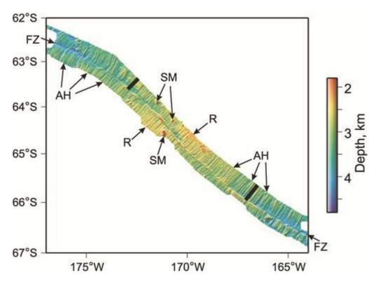
Caption: Multibeam acoustic swath bathymetry image of seafloor topography from the southeastern Pacific. 'R' denotes mid-ocean ridge, 'FZ' fracture zone, 'SM' seamount, and 'AH' abyssal hill. Note that the abyssal hills form a fabric whose grain is parallel to the ridge. From J. A. Goff et al., "The contributions of abyssal hill morphology and noise to altimetric gravity fabric," Oceanography 17, 24-37, 2004.
