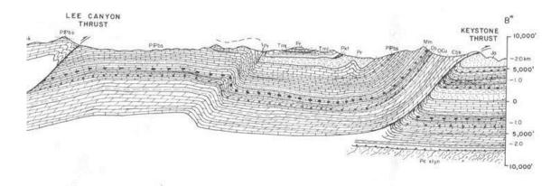
Caption: East-west cross section from just west of Las Vegas, Nevada, showing the Keystone Thrust Sheet, interpreted here as a gigantic gravity slide feature.
