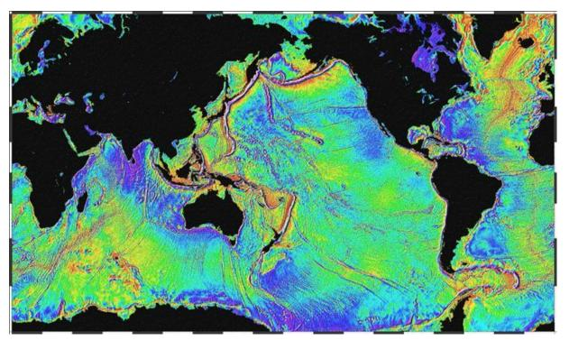
Caption: Free-air gravity anomaly map of the world's oceans. This map was generated from geoid height measurements from 4.5 years of measurements by the U.S. Navy's Geosat satellite and 2 years of measurements by the European Space Agency's European Remote Sensing ERS-1 satellite.
