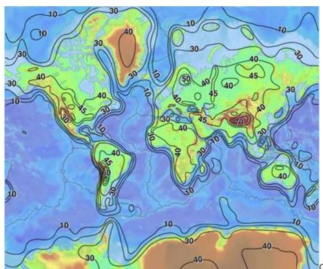
Caption: Contour map of the thickness of the Earth's crust developed from the CRUST 5.1 model (Mooney et al., 1998). The contour interval is 10 km with the additional 45 km contour for greater detail on the continents. There is close agreement between observed and predicted Love waves (surface shear waves) with a period of 40 s. These phases are primarily sensitive to the shear velocity and density structure in the upper 40 km. (http://earthquake.usgs.gov/research/structure/crust/index.php)
