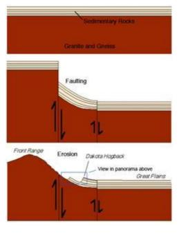
Caption: Sketch showing in three steps how the Front Range has been uplifted along a major fault, or a series of faults. Uplift west of the main fault has exhumed granites and gneisses from deep in the crust, and any sedimentary layers on top of them have since been removed by erosion. East of the fault systems the sediment layers have survived.
