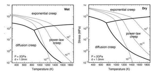
Caption: Deformation mechanism map of wet and dry olivine as functions of stress and temperature at P = 2GPa and grain size of 1.0 mm.
