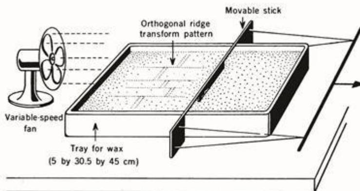
Caption: (Above) Experimental apparatus. A tray of melted paraffin was cooled with a variable-speed fan until a film of solidified wax formed between one end of the pan and a movable stick. The stick, representing the edge of a moving
